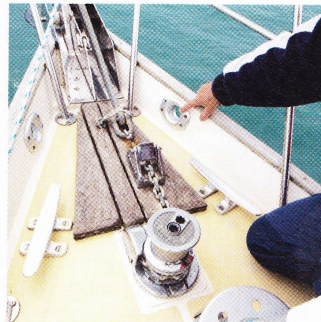
Her foredeck has a powerful windlass, twin roller, chunky cleats and captive fairleads
